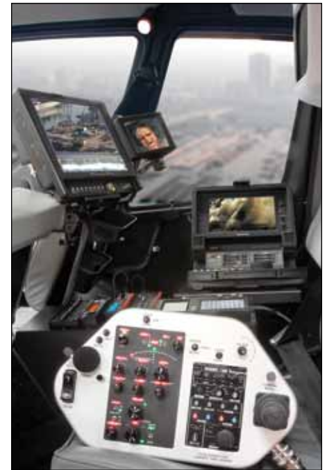
A laptop console consolidates all of the camera controls and functions for ease of use.
