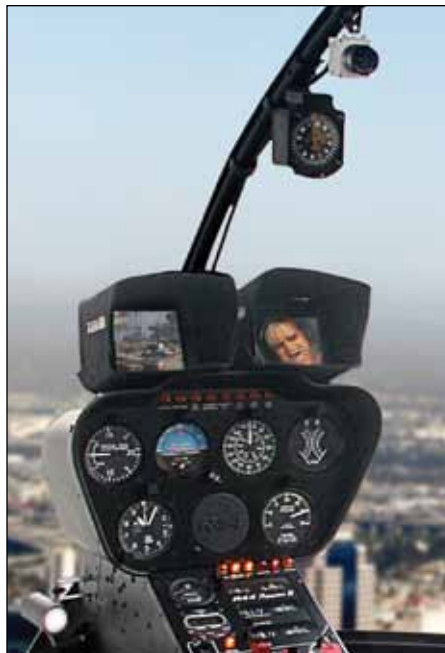
Forward cabin has two monitors to view images from any of the helicopter's cameras and on-air broadcast.
